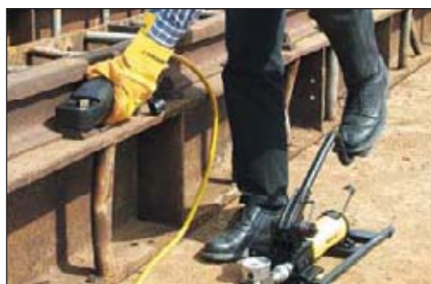
◀ Easily removing rusty nuts during railroad construction is just one of many application examples for the Enerpac Nut Cutters.
