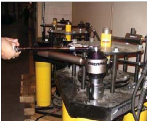
◀ Enerpac Reaction Bar Torque Multiplier E393 used to manually torque bolts up to 4340 Nm.
